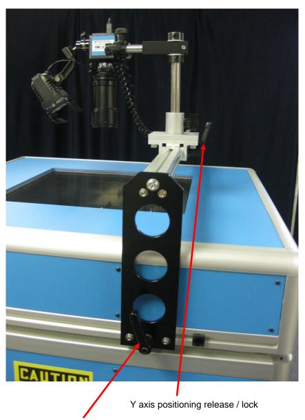
X axis positioning release / lock (shown 1 of 2 - not shown is located on the opposite end of the cover)
