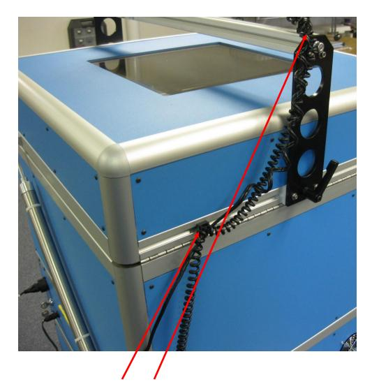
Use plastic cable ties to secure the cables
