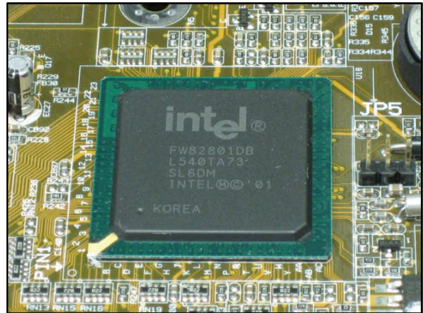
Figure 10: BGA installed on a motherboard
